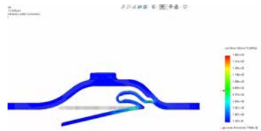
Prototype 2 - Version 4 - Yield Strength Simulation
