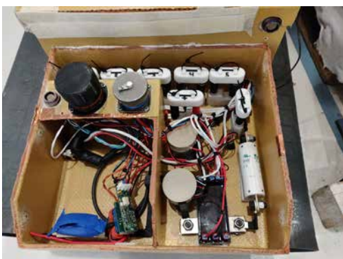
Abb. 4: Energymeter Box (EMB) Verdrahtung
