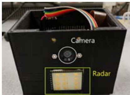
Abb. 2 Housing with sensor and camera
