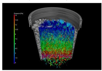
ting point of simulations of the water permeability. Shown in the beaker are the spherical zeolite particles, the flow lines with colour-coded velocity and the distribution of pressure levels.
