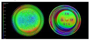
Nominal-actual comparison of the cap of a water bottle. The orthogonal deviation between the two geometries is colour coded.
