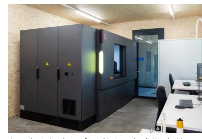
rior and exterior shape of an object can be digitised with metrological accuracy. The short acquisition time for CT measurements also enables the inspection of dynamic processes to track the changes inside an object in 3D. LuCi is capable to inspect a wide range of different materials starting from wood, aluminium, steel or even denser materials. Besides technological samples also biological samples such as fruits, vegetables, cheese, or biological tissues can be inspected.
