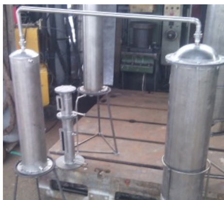
Figure 7: Reactors for PEEK cycling for resin recovery
