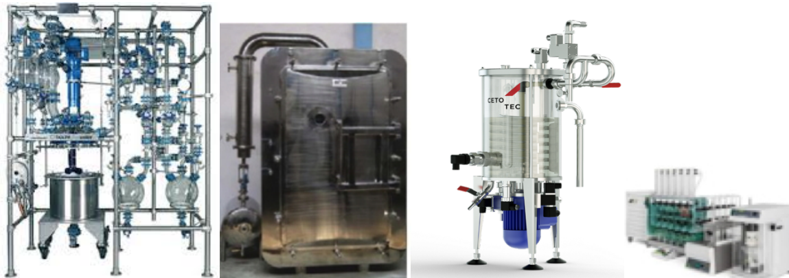
Figure 6: Dean-Stark trap (from left to right) with distillation and condenser system, vacuum dryer, a fermenter reactor and a Soxhlet still
