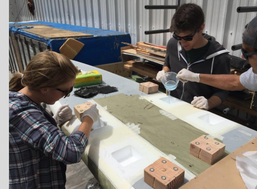
Applying epoxy for the insert assembly at Ding King
