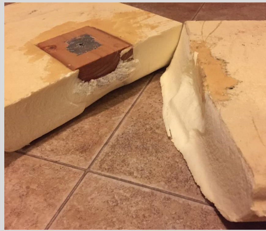
Failure in foam structure of surfboard blank test specimen
