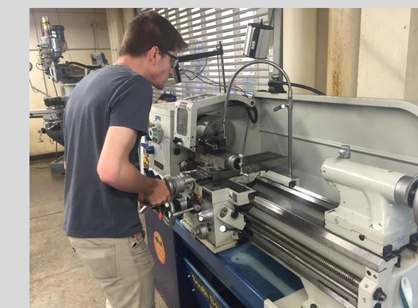
Spencer using the lathe to face the joint pins
