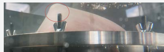
Figure 6: Punctured + untreated foetal membrane while running the kicking sequence. An extension of the foetal membrane through kicking is visible (see red circle).
