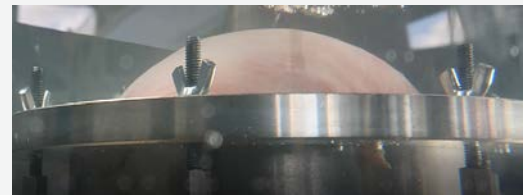
Figure 5: Punctured + untreated foetal membrane on the ex-vivo model inflated to an 40mm bulge before starting kicking sequence.
