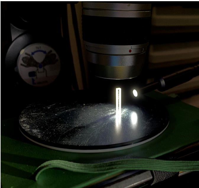
Figure 2: Analysis of glass capsule after drop test.
