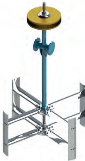
Abb. 1: H-Darrieus Turbine EVG-005 der New Energy Corporation
