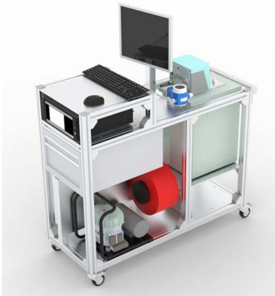
Fig. 1: Rendering of the mobile pressure and temperature sensor calibration module (PTCM)
