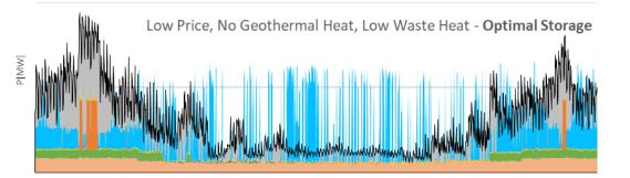
■ Discarge Storage ■ Air Heatpump ■ Gas Heater ■ Gas CC CHP ■ Biomass Heater ■ Biomass CHP ■ Geothermal ■ Industrial Waste Heat □ demand
