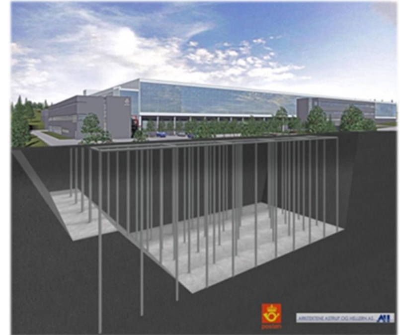
BTES at Postterminal building, Lørenskog, Norway
