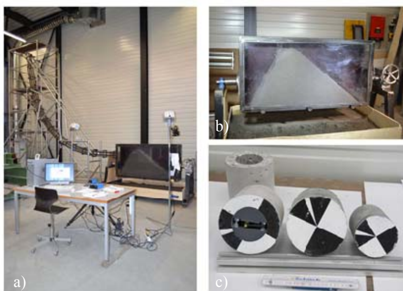
Fig. 1 Experimental equipment for small scale quasi-2D-impact tests, a) testing facility, b) construction box with model embankment, c) impact bodies
