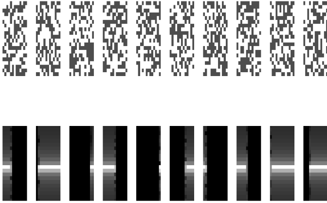
Fig. 2. Noise power patterns of size 13 \times 20 . White colored time/frequency slots are subject to intense noise power and black colored slots are subject to weak noise. Above: artificially generated patterns with 10 dB difference in noise power. Below: patterns resulting from narrowband interference partially overlapping in time.
