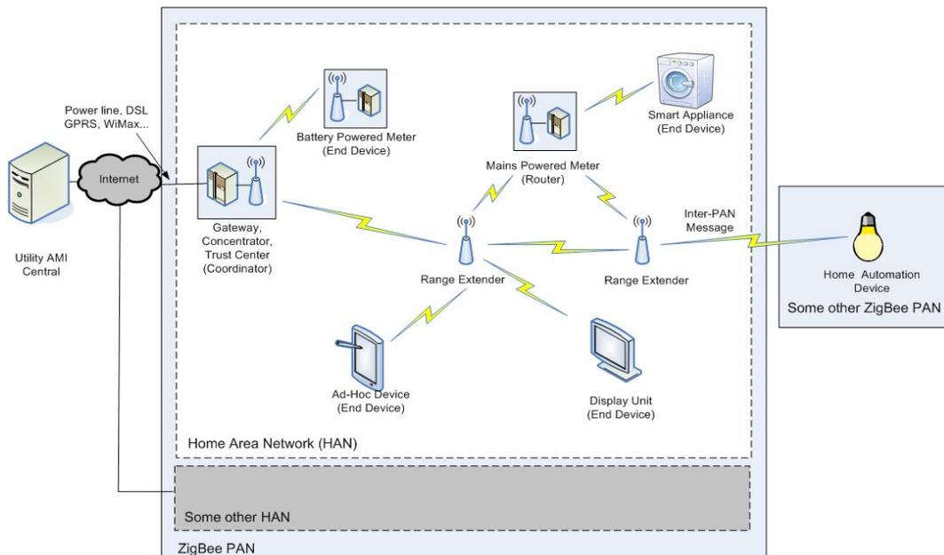
Figure 4: Example of a ZigBee Smart Energy Network
