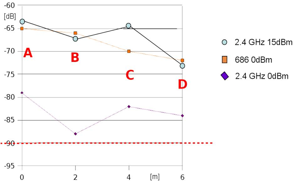
**Figure 2: Example of 2.4 GHz transmission through a 40 cm concrete wall with 3 different transmitters. Red dotted line indicates the "critical Area", levels below -90 dB are not sufficient for reliable communication.**
