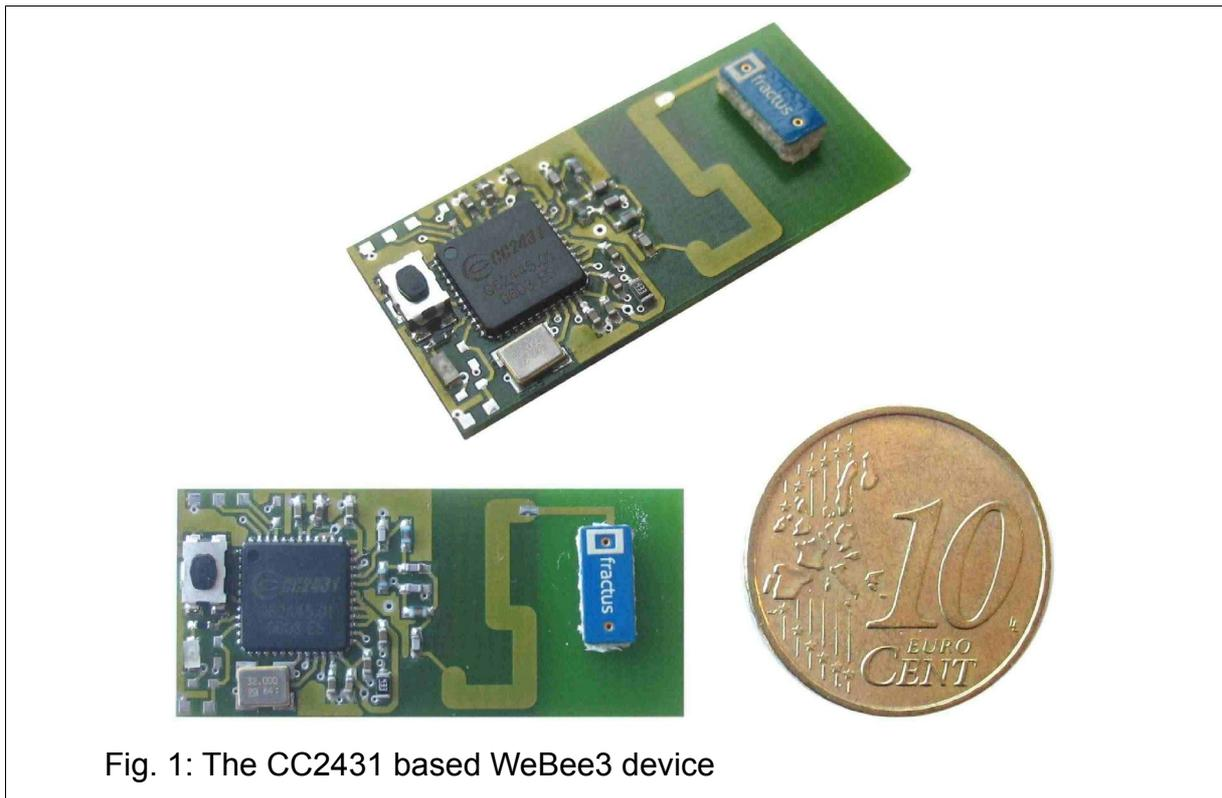
Fig. 1: The CC2431 based WeBee3 device
