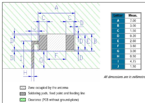
Fig. 4: Antenna PCB layout detail
