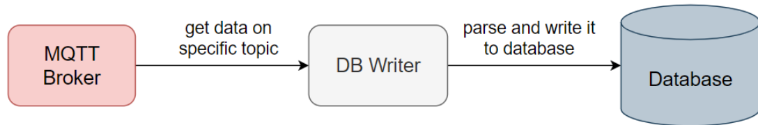
Figure 3: Diagram of the DB Writer object
