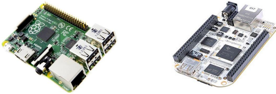
Figure 2. Raspberry Pi 1 Model B+ and BeagleBone Rev A6 single board computers
