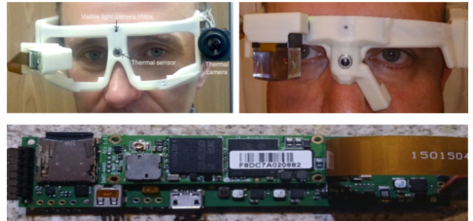
Fig. 3. The eGlasses prototypes with three sources of potential medical data: the visible-light imaging camera, the thermal camera, and the thermal sensor. Below electronic board from the side panel of the eGlasses is presented.
