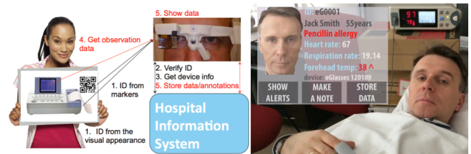
Fig. 2. a) Interaction of smart glasses with a HIS using data from the identified medical device connected to the patient (simulated hospital environment). b) An example of possible data presentation on the near-to-eye display of the smart glasses
