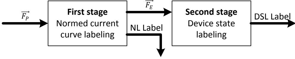
**Figure 1 Schema of the two stage cascading NIALM algorithm. The first stage detects events which are then further analysed by the second stage to obtain device specific information.**
