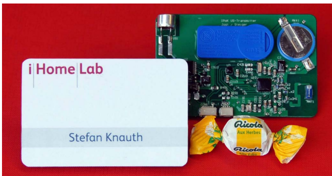
Fig. 2. Mobile Node: a visitor badge. The badge comprises a PCB equipped with a TI-CC2430 System-on-Chip including an IEEE802.15.4 transceiver, a chip antenna, a rechargeable lithium coin cell, an accelerometer, the ultrasound transducer and a driver for the latter.
