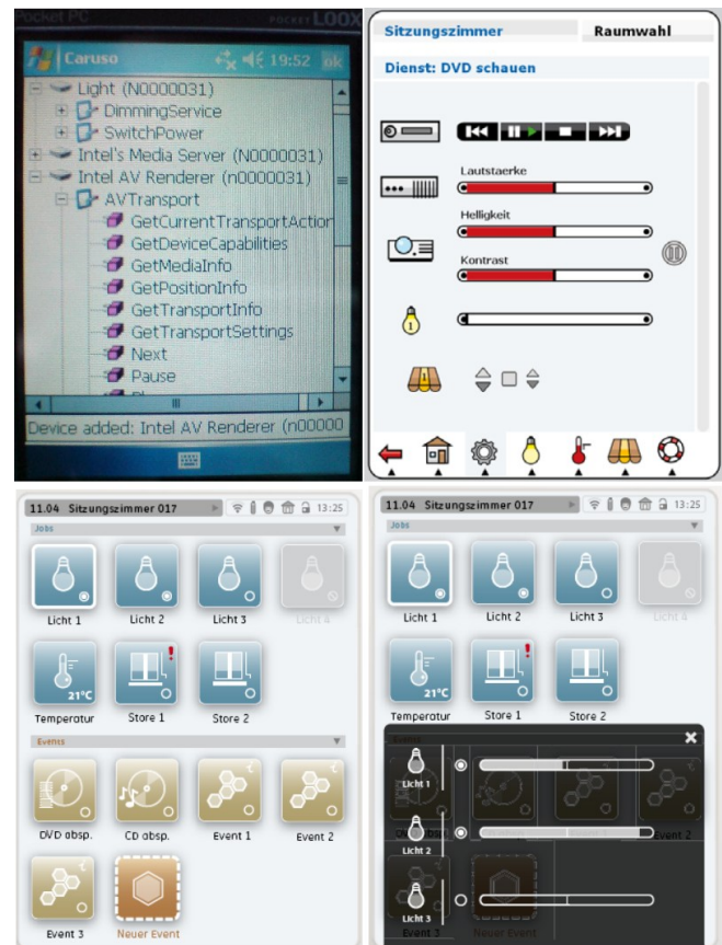
Fig. 2. Upper row, left: UPnP Control Point Prototype, right: Generated SVG Prototype for service "Watch DVD". Lower row: Design Studies
