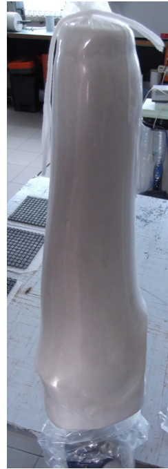
negative form of the prosthesis with PVA-coat
