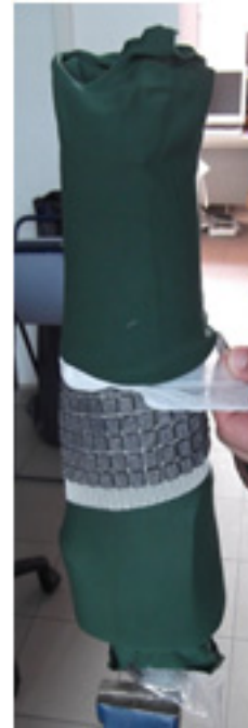
Coating of a further, stable textile stocking and the PCM-sleeve
