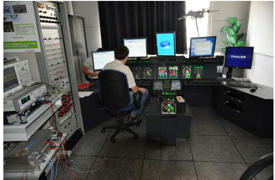
CDS test bench (Thales Avionics)
