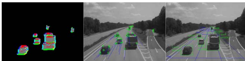
Figure 2: Video Content Analysis: object extraction (left), object tracking (centre), object classification (right)
