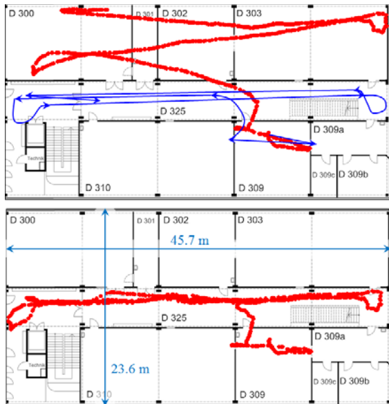
Figure 4 (top) IMU based navigation with heading deviation induced by a parasitic magnetic field (top). The same data corrected with the heading information obtained from the image correlation technique (bottom). The real path (for both cases) is shown as blue arrows (top).
