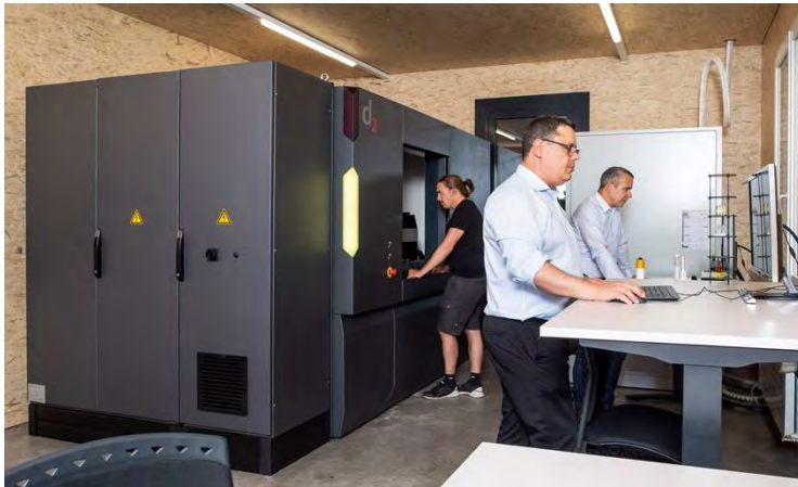
Picture: Lucerne CT Imaging (facility): "Luci" is a computer tomograph measuring 3.5 x 2.0 x 2.5 meters and weighing about 11 tonnes. Department T&A, Hochschule Luzern, 2025
